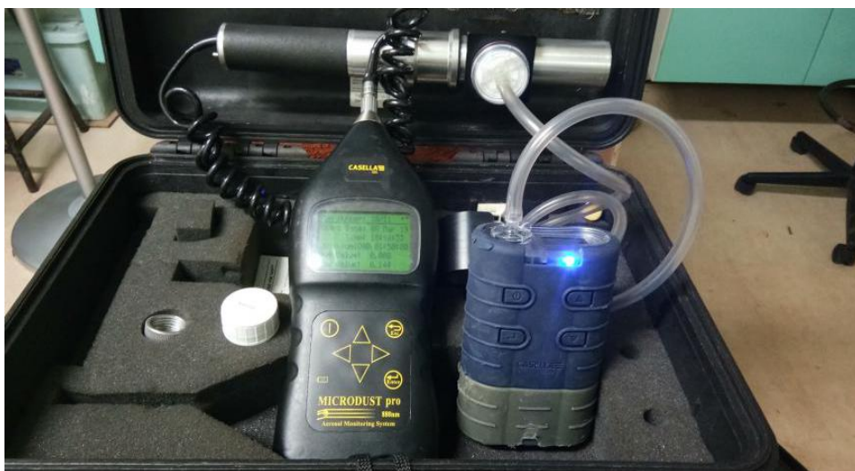
Figure 3.2 Dust Detective / Portable Air Sampler
