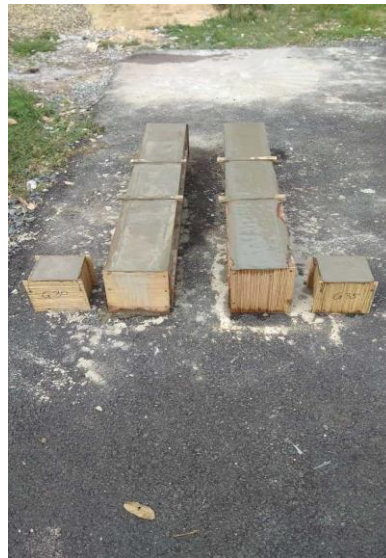
Figure 4: 0% C RCB casting
