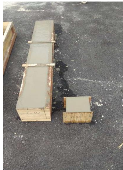
Figure 5: 10% SCPWP RCB casting
