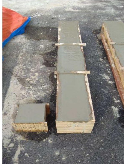
Figure 6: 10% SCBWP RCB casting
