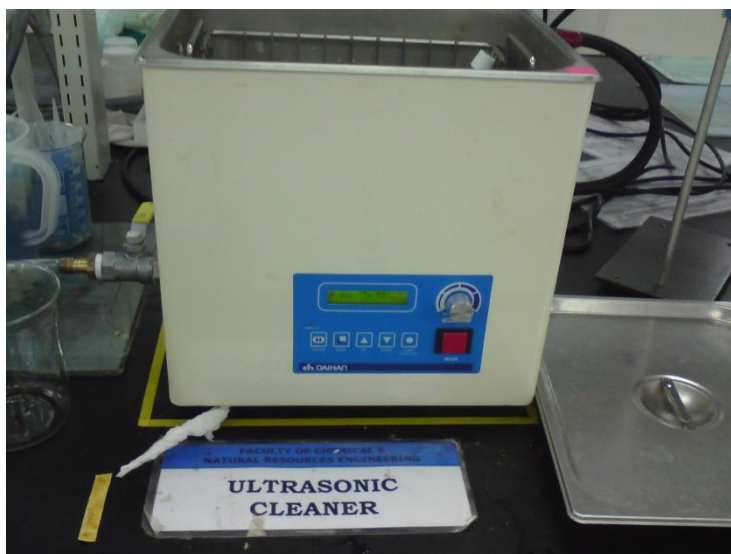
Figure 3.2 DAIHAN Digital Ultrasonic Cleaner
