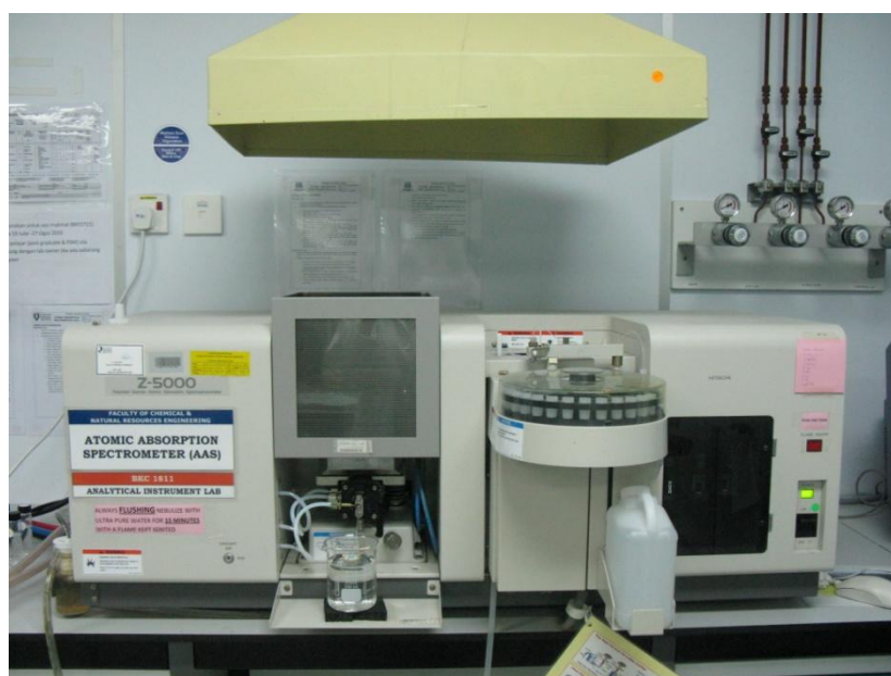
Figure 3.3 HITACHI Z-5000 Polarized Zeeman Atomic Adsorption Spectrometer
