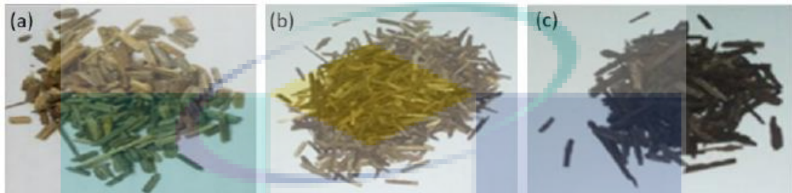
Figure 2.1 Images of oil palm frond at (a) raw, (b) torrefied at 240 °C and (c) torrefied at 300 °C
