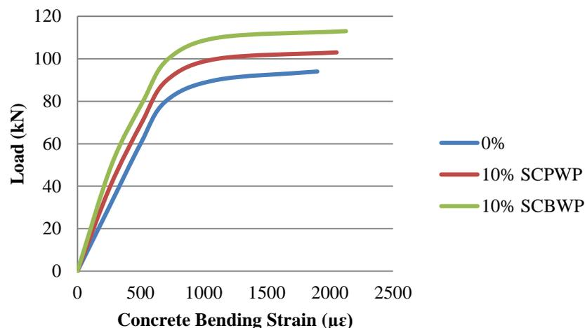
**Figure 4.** Load-strain curves for beam with full shear reinforcement (SS=100 mm)
