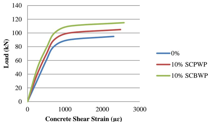
**Figure 7.** Load-strain curves for beam with full shear reinforcement (SS=100 mm)
