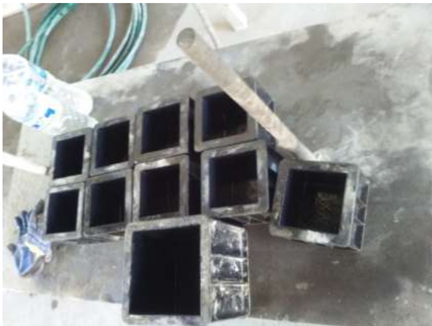
Figure 3.17 Mould size 100mm x 100mm x 100mm
