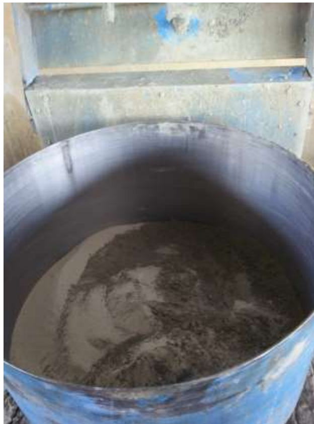
Figure 3.15 Cement and Fine Material in Mixer
