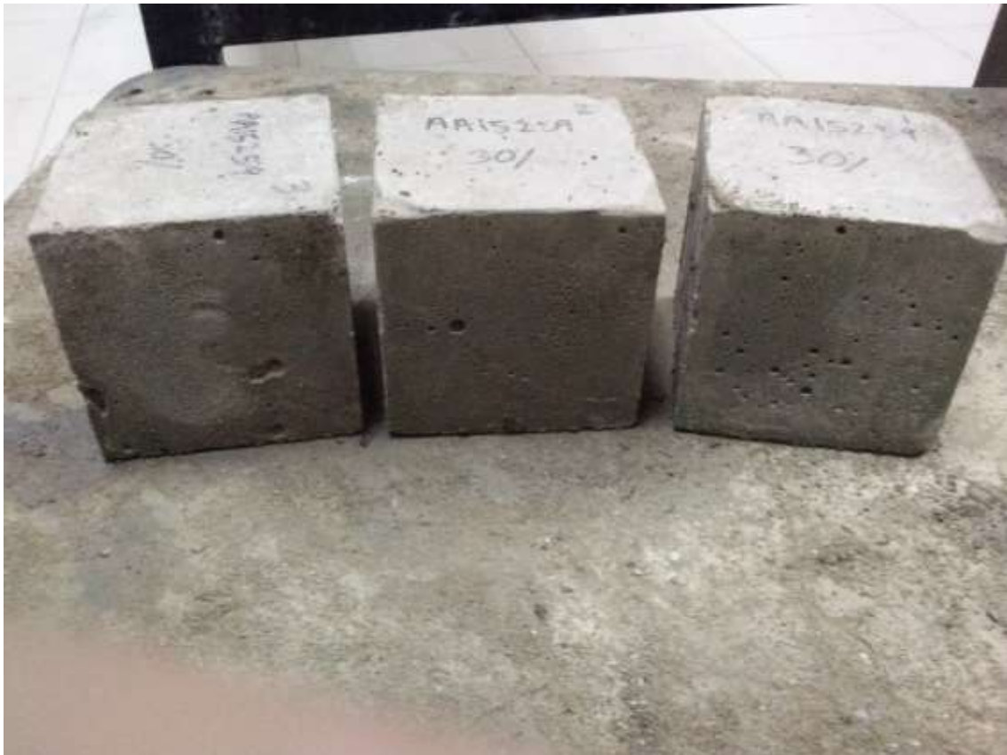
Figure 3.24 Foam Concrete Ready for Compression Test
