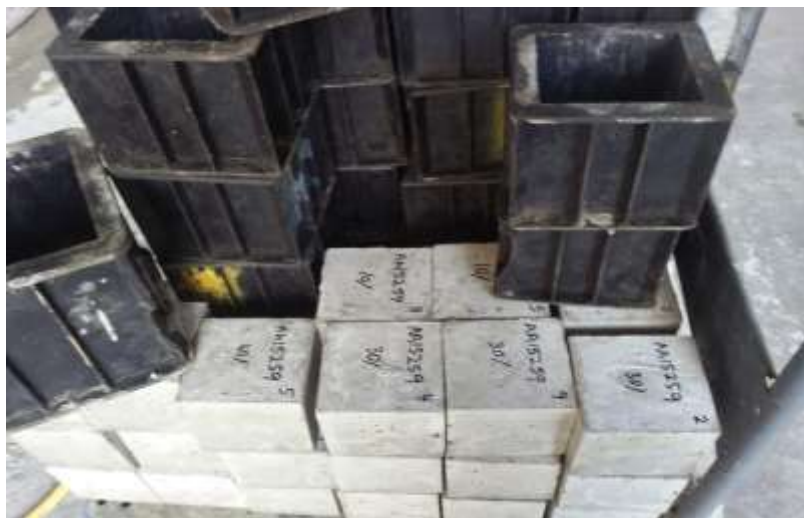
Figure 3.21 Remove Foam Concrete from Mould
