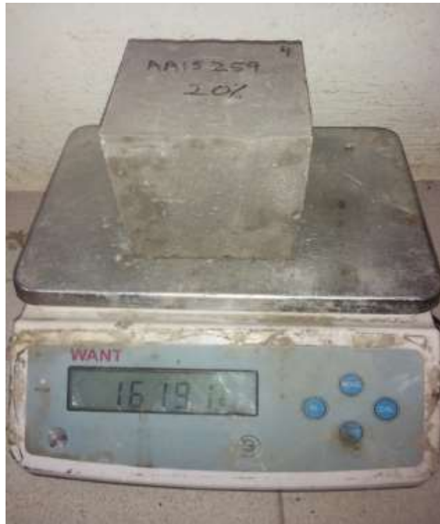
Figure 3.22 Weighted Hardened Foam Concrete
