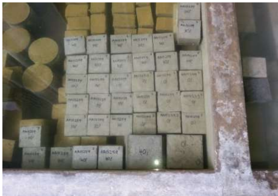
Figure 3.23 Water Curing Process
