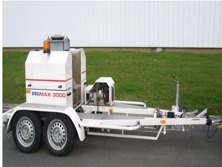
Figure 2 : falling weight deflectometer
