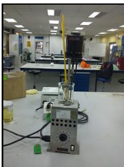
Figure 3. 2 Dropping point test apparatus
