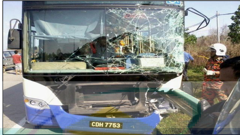
Figure 4.53 A metal beam punctured through the rapid Kuantan bus at KM 13 Kuantan-Pekan, Pahang
