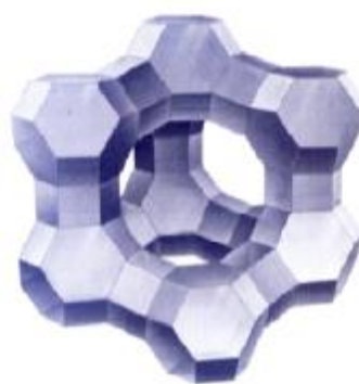
Figure 2.12: Zeolite molecular sieve type X
