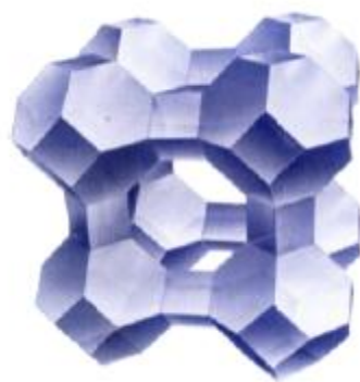
Figure 2.11: Zeolite molecular sieve type A
