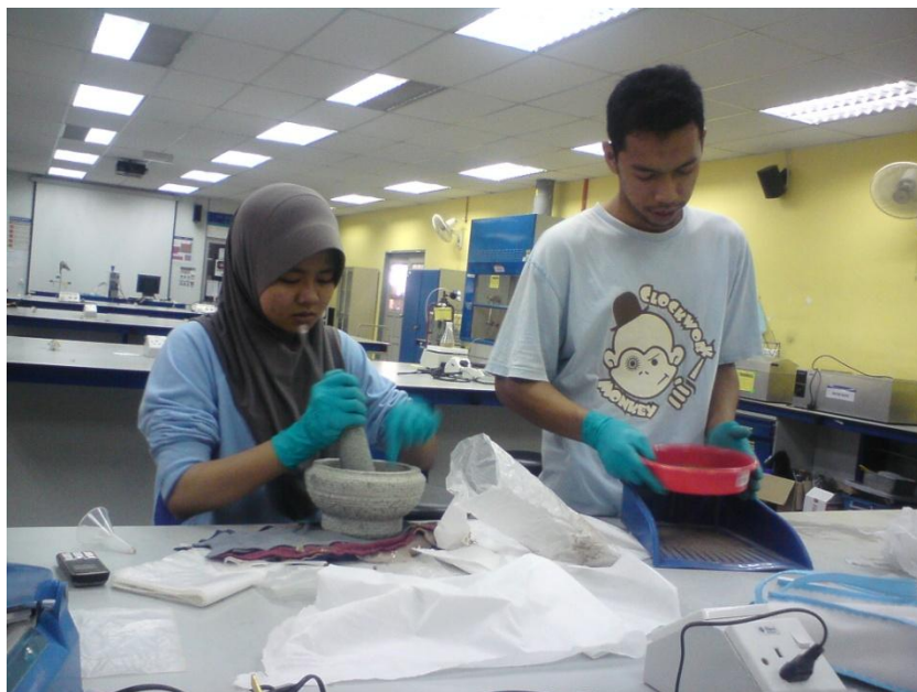
Figure B.4 Sample pulverized and sieved
