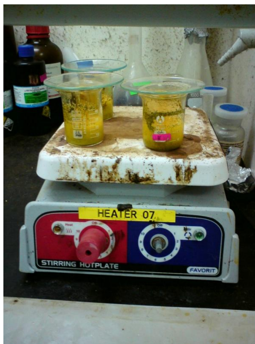
Figure B.5 Sample digestion
