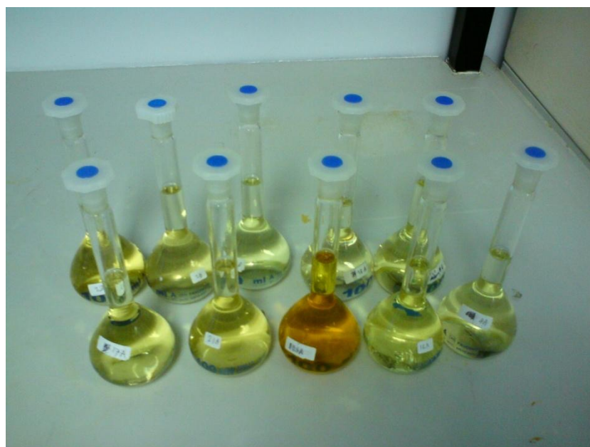
Figure B.6 Diluted samples and ready for AAS analysis
