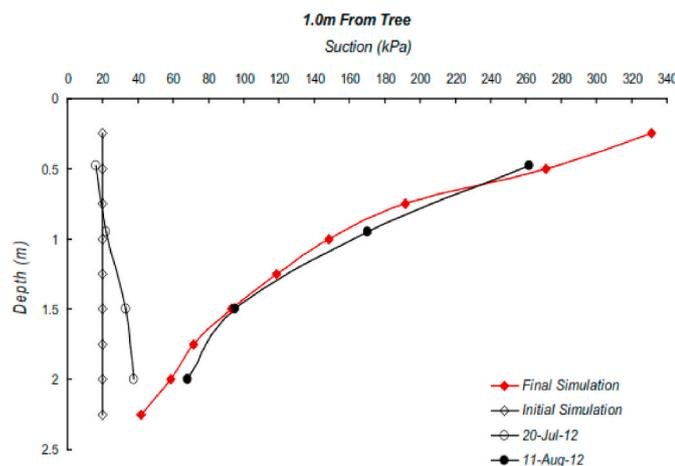
**Fig. 10.** Simulated (period of time 21 days) and measured matric suction profile. From 20<sup>th</sup> July 2012 to 11 th August 2012 at 1 m from tree.
