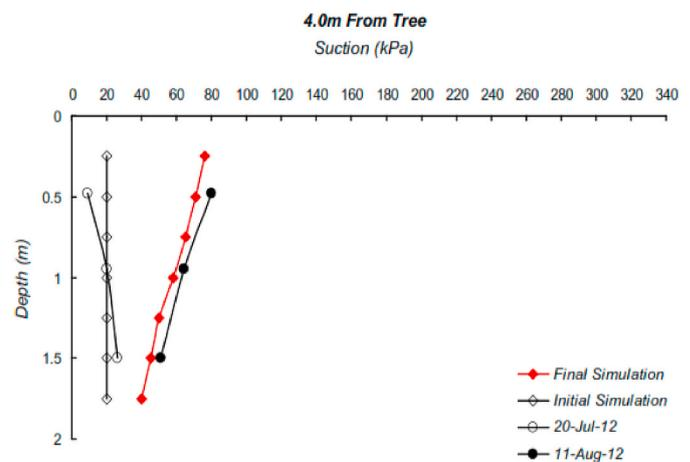
**Fig. 12.** Simulated (period of time 21 days) and measured matric suction profile. From 20<sup>th</sup> July 2012 to 11 th August 2012 at 4 m from tree.
