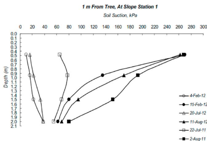
Fig. 3. Progressive development of matric suction during the drying periods at 1 m from tree.
