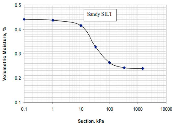
Fig. 7. The soil-water characteristic curves (SWCC) of the residual soil.
