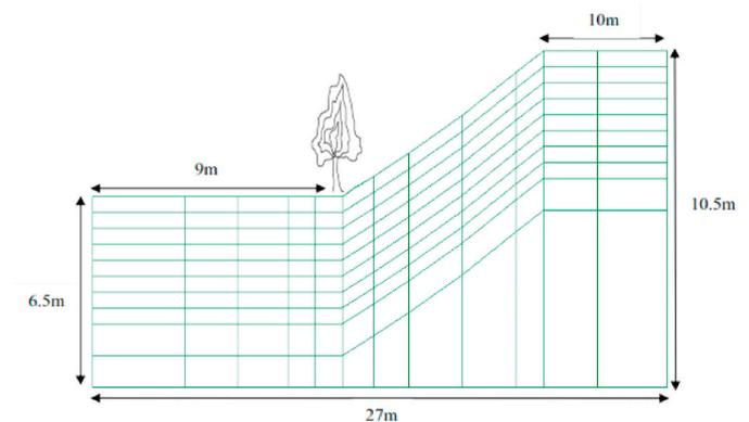
**Fig. 13.** Finite element mesh of measured slope geometry with tree at toe of slope.
