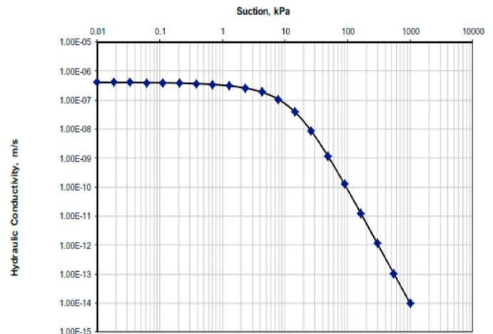
Fig. 8. Hydraulic conductivity function with responds to matric suction of the residual soils predicted by using Van Genuchten's model (1980).
