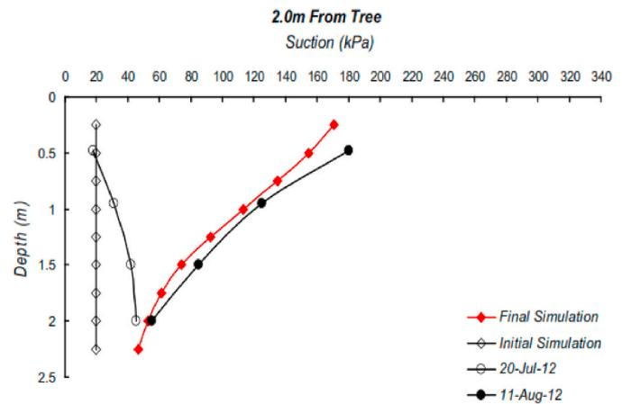
**Fig. 11.** Simulated (period of time 21 days) and measured matric suction profile. From 20<sup>th</sup> July 2012 to 11 th August 2012 at 2 m from tree.
