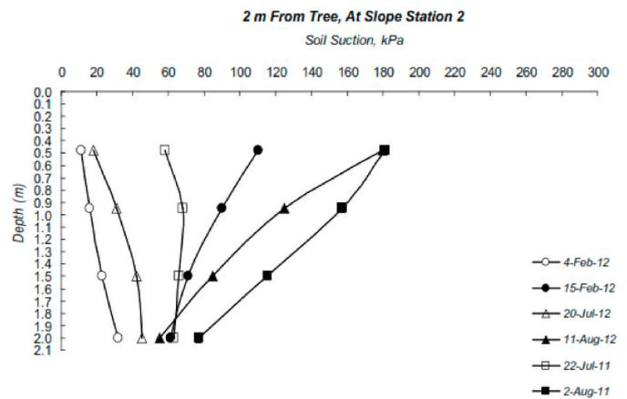
Fig. 4. Progressive development of matric suction during the drying periods at 2 m from tree.
