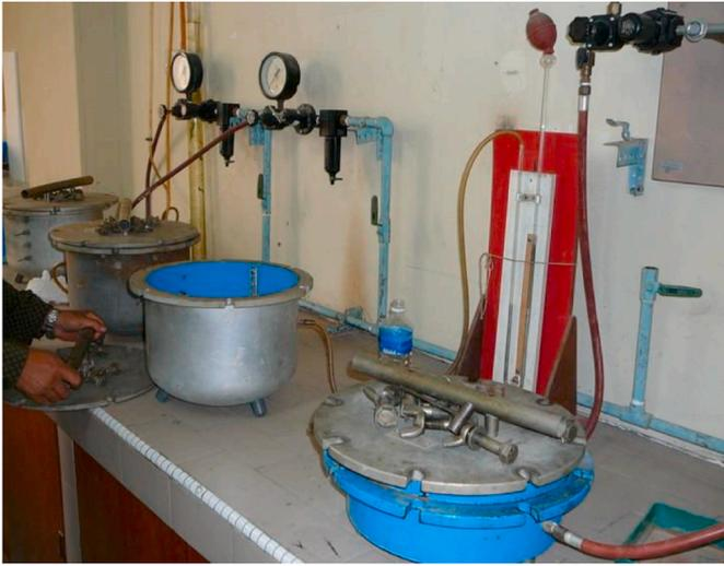
Fig. 2. Pressure plate extractor test setup in Universiti Putra Malaysia.
