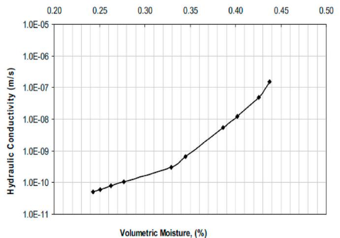
Fig. 9. Hydraulic conductivity function with responds to volumetric water content of the residual soils predicted by using Van Genuchten's model (1980).
