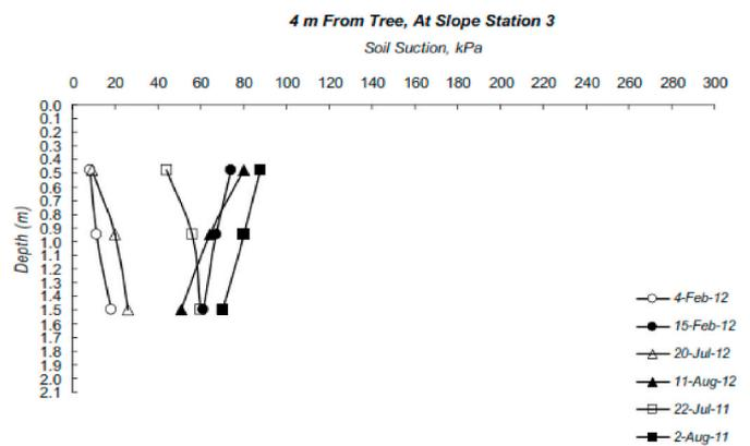
Fig. 5. Progressive development of matric suction during the drying periods at 4 m from tree.
