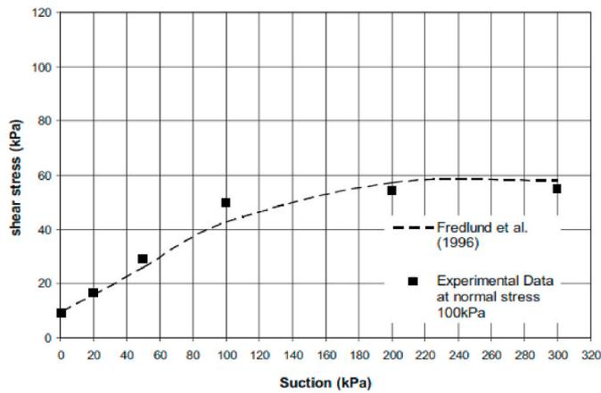
Fig. 6. Comparison of nonlinear failure envelope for the soil at study area.
