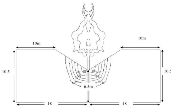
Fig. 14. Comparison of matric suction contour (kPa) generated within the vicinity of *Acacia Mangium* tree at toe of slope (a) numerical simulation. (b) actual field measurement results.
