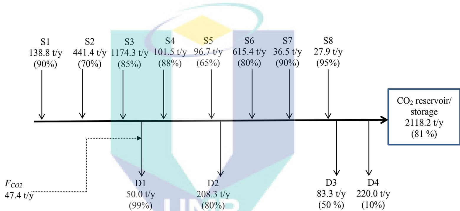
**Figure 5.4:** Optimal network for CO<sub>2</sub> Total Site Scenario 2
