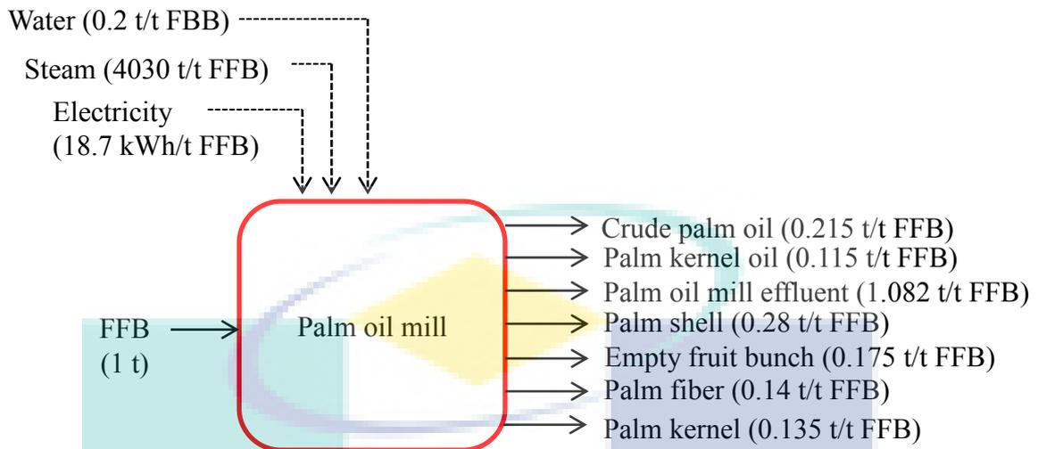
**Figure 4.6:** In and out diagram for palm oil mill (Kasivisvanathan *et al.*, 2012)
