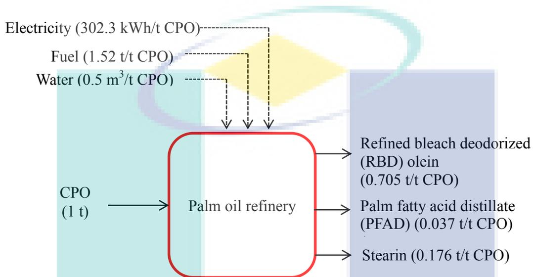
**Figure 4.7:** In and out diagram for palm oil refinery (Haslenda and Jamaludin, 2011)
