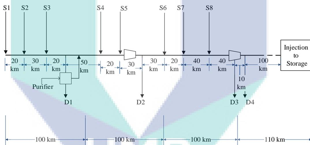
**Figure 6.5:** CUS design network with purifier and installation of compressor
