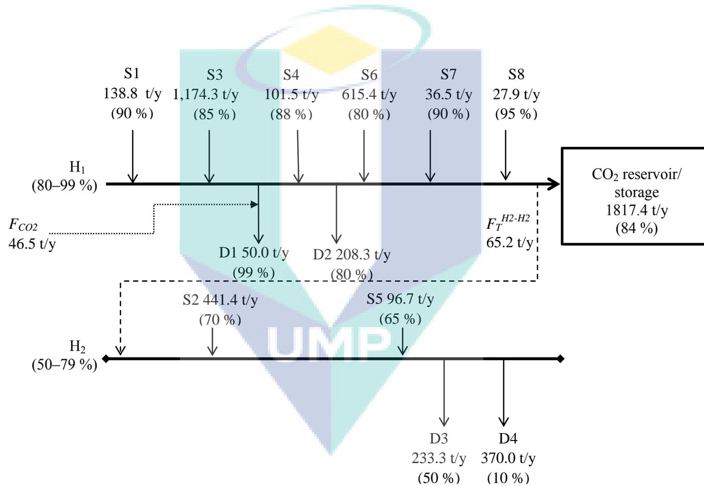
Figure 5.6: Optimal network for CO<sub>2</sub> Total Site Scenario 4
