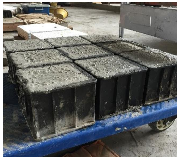
Figure 2 Plastic mould for preparing (150x150x150mm) cubes
