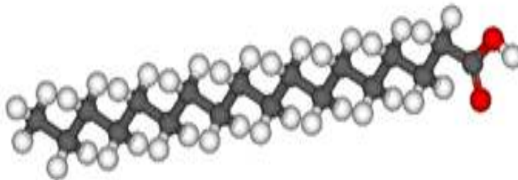
Figure 2.5: 3-D molecular structure of Stearic Acid
