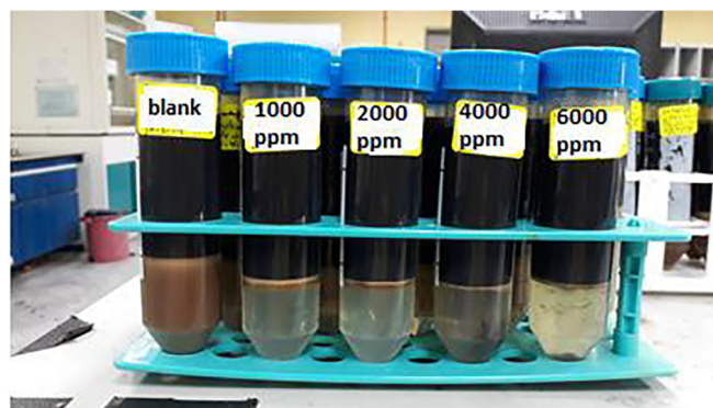
Fig. 7. Demulsification photos for W/O emulsions.
