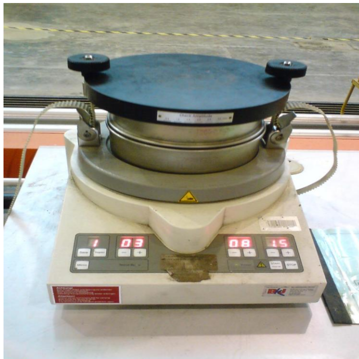
Figure 3.3: Sieving process of the bagasse to attain 0.5 mm size of mesh powder
