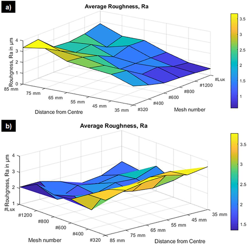
Fig. 6. Surface roughness measured from inner to outer side of the tile surface subjected to a) triangular distributed load and b) uniform distributed load.
