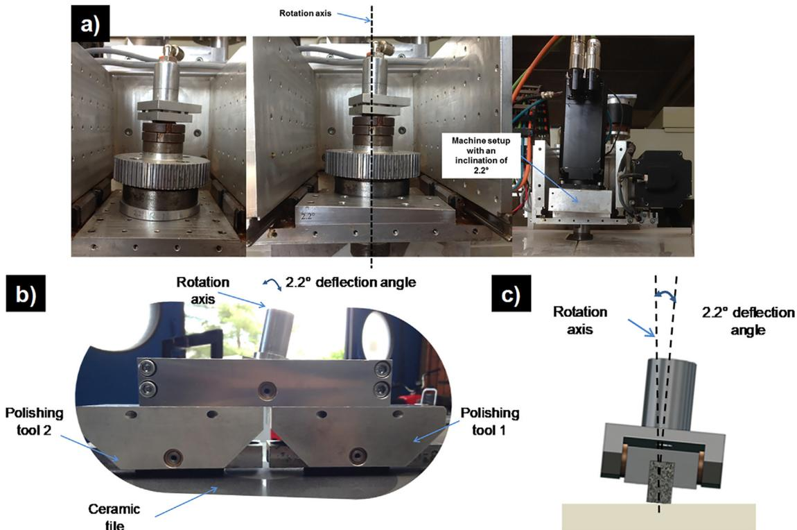
Fig. 2. Tribometer and polishing head with two polishing tools. (a) Installation of 2.2° inclined armatures on the tribometer; (b) Deflection of the polishing head; (c) Illustration of the deflected polishing tool.
