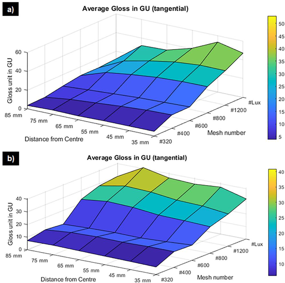
Fig. 5. Gloss Unit measured in direction tangential to the tile's radius subjected to a) triangular distributed load and b) uniform distributed load.
