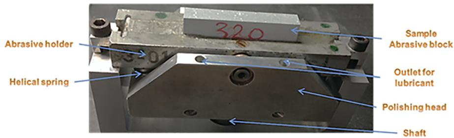
Fig. 1. A sample of abrasive block fixed on its holder as a polishing tool (fickerts).
