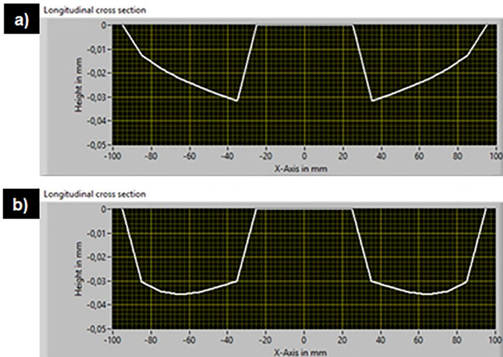
Fig. 7. Wear depth of the polished surfaces measured from the tile center after being subjected to a) triangular distributed load and b) uniform distributed load.
