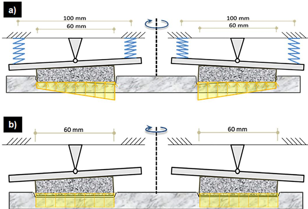
Fig. 3. Polishing head configuration against ceramic tile during the experiment (a) triangular distributed load (with helical springs attached) (b) uniform distributed load.
