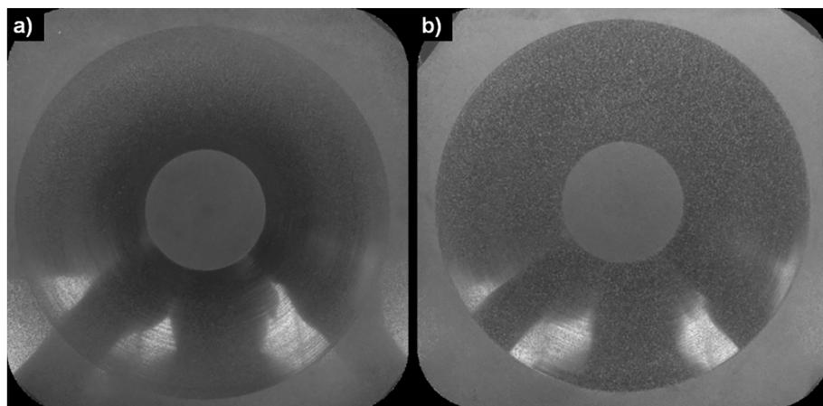
Fig. 9. Scratching score and the development of gloss on the ceramic tile being subjected to a) triangular distributed load and b) uniform distributed load.
