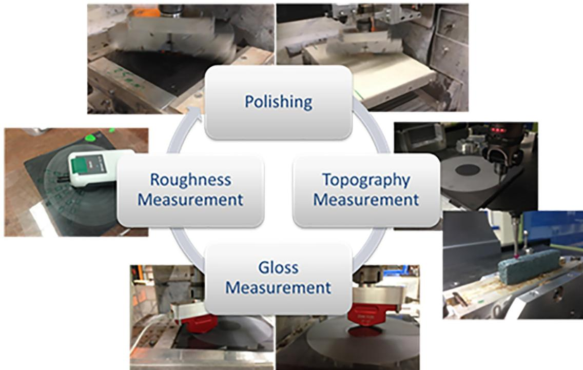
Fig. 4. Experimental sequence and cycle [6].
