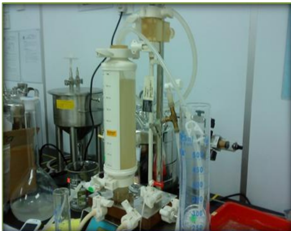
Figure 3.6: Membrane system for separation process
