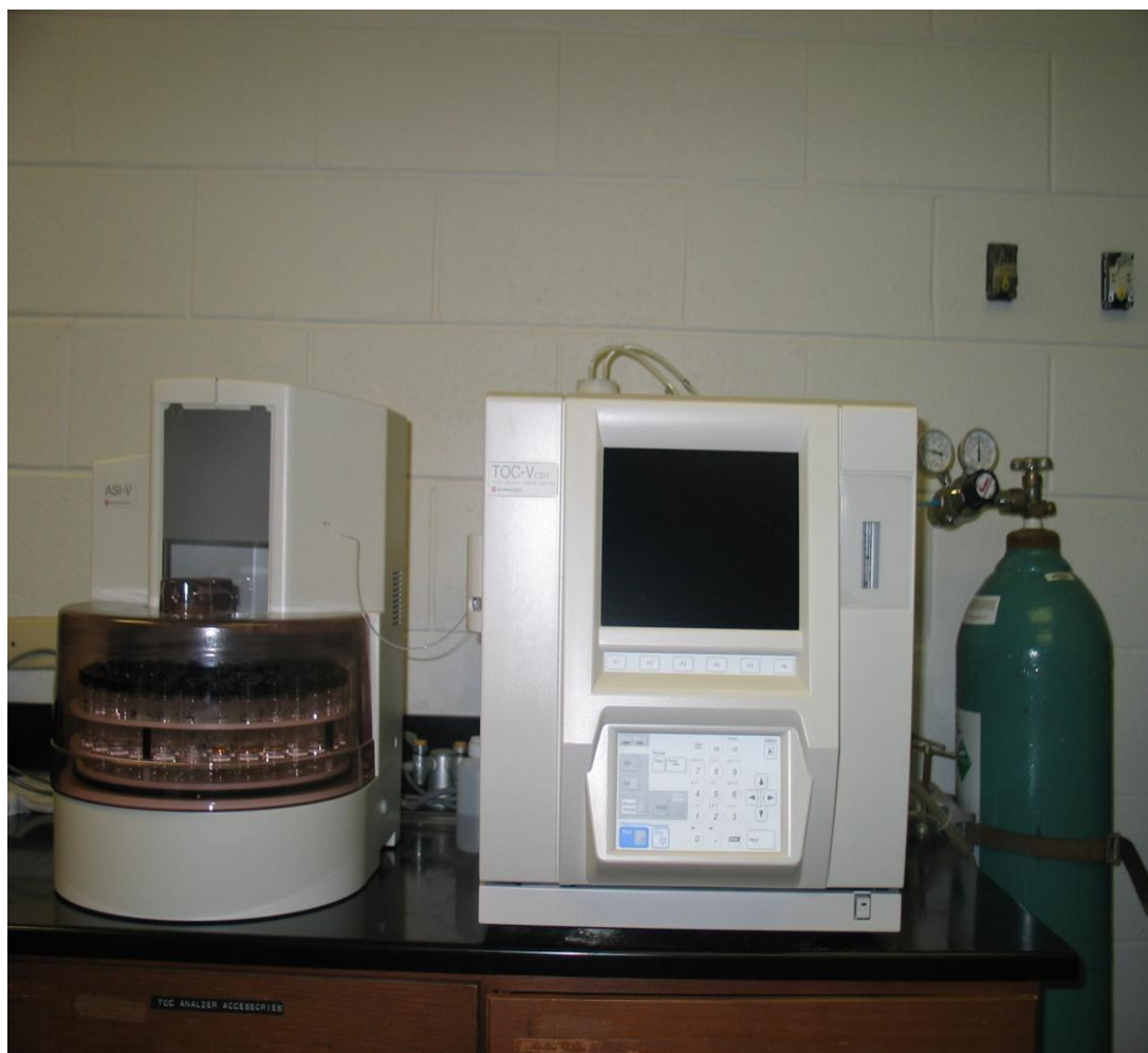
Figure 3.8: Total organic carbon analyzer
