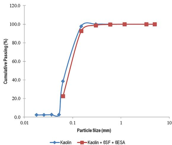
Fig. 10 – PSD curve of untreated kaolin and treated kaolin with an optimum dosage of stabilizers (6% SF & 6% ESA).
