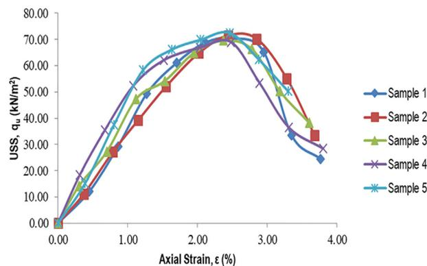
Fig. 11 – Stress–strain graph of the kaolin treated with 6% of SF and 6% of ESA content.
