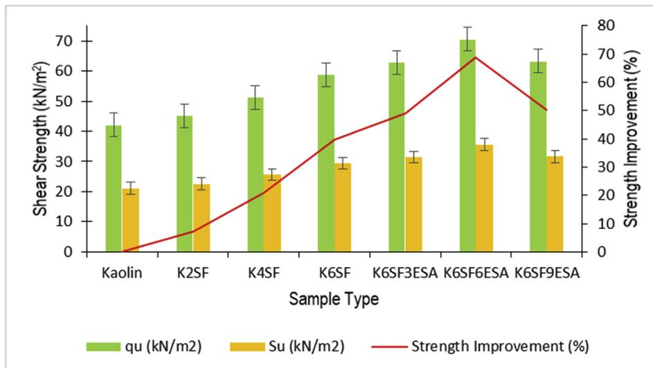
**Fig. 5 – Relationship between type of samples with sample strength (kN/m<sup>2</sup>) and strength improvement (%).**
