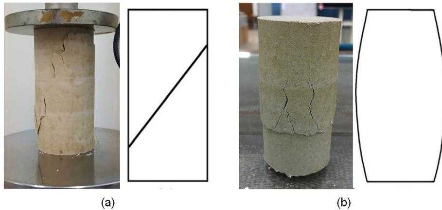
**Fig. 12 – Compacted soil sample of (a) shear failure (b) bulging failure.**
