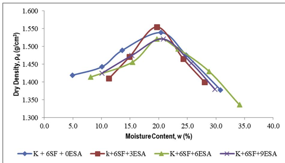
**Fig. 7 – Compaction curve of kaolin admixed with 6% SF and various percentage of ESA content (%).**
