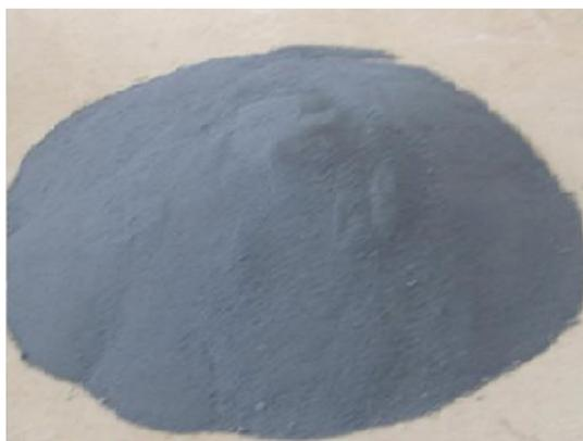
Fig. 2 – Grey colour-densified Silica Fume.
