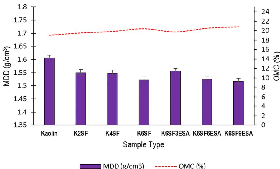
**Fig. 8 – The correlation between MDD (g/cm<sup>3</sup>) and OMC (%) of the kaolin sample admixed with 6% of SF and various percentage of ESA content (%).**
