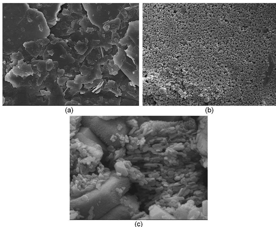
**Fig. 13 – FESEM images under  $\times 10,000$  magnification of (a) untreated kaolin, (b) SF, and (c) ESA.**
