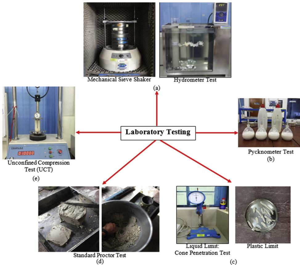
Fig. 4 – Laboratory test conducted (a) Particle Sieve Analysis (b) Specific Gravity Test (c) Atterberg Limit Test (d) Standard Compaction Test (e) UCT.
