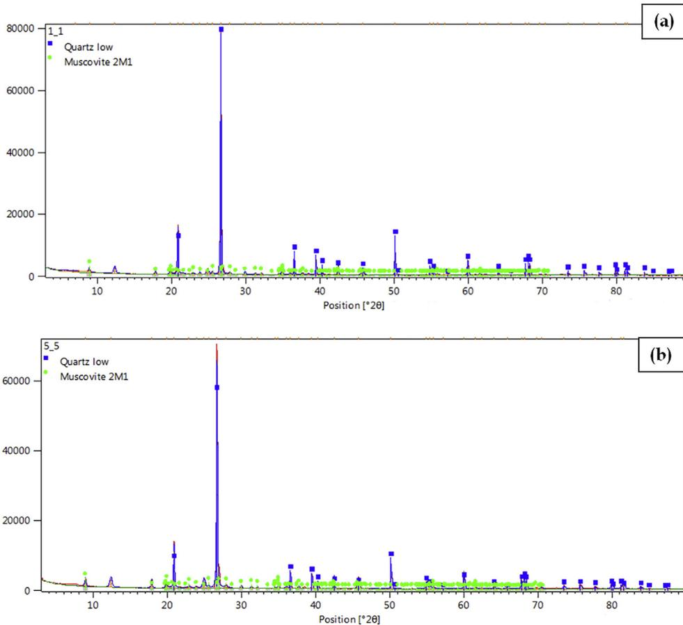
**Fig. 9 – The XRD results for (a) untreated kaolin (b) treated kaolin with 6% of SF and 6% of ESA content.**
