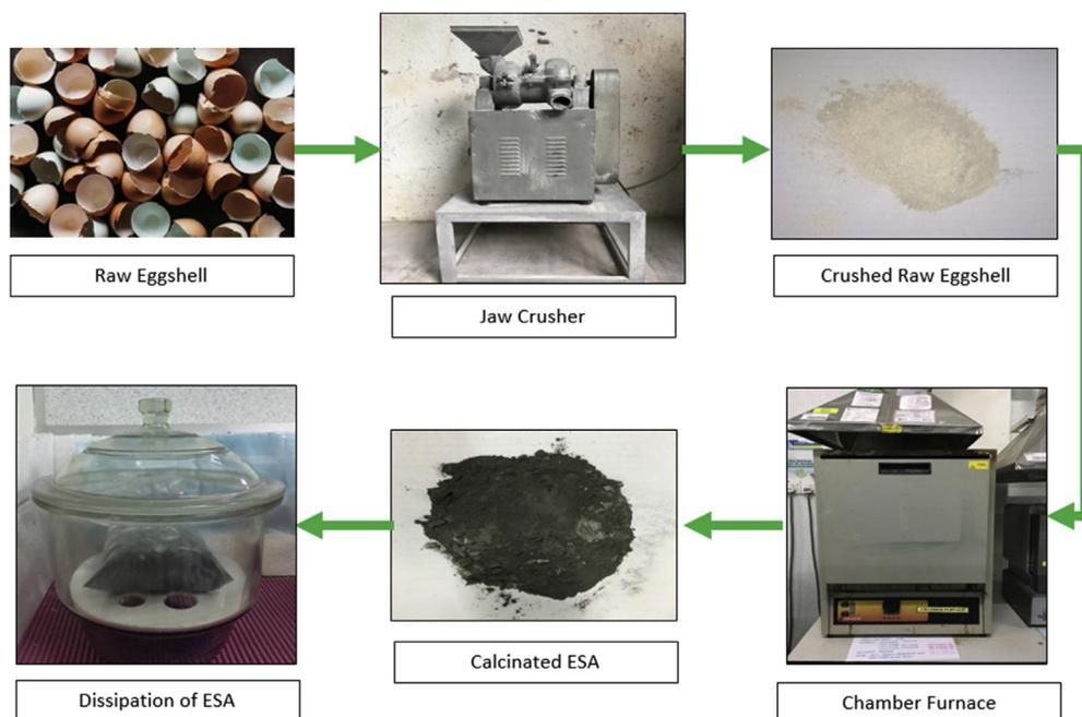
Fig. 3 – Sample preparation of the ESA.
