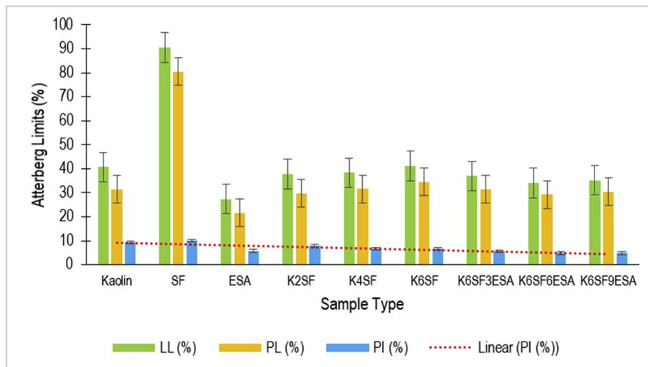
**Fig. 6 – Relationship between types of a sample with sample Atterberg limits (%).**
