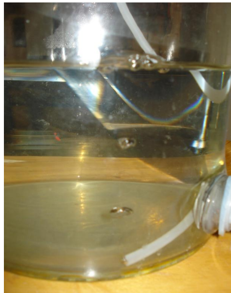
Figure 3.15: Bubbles formed in 20 liter Displacement Bottle
