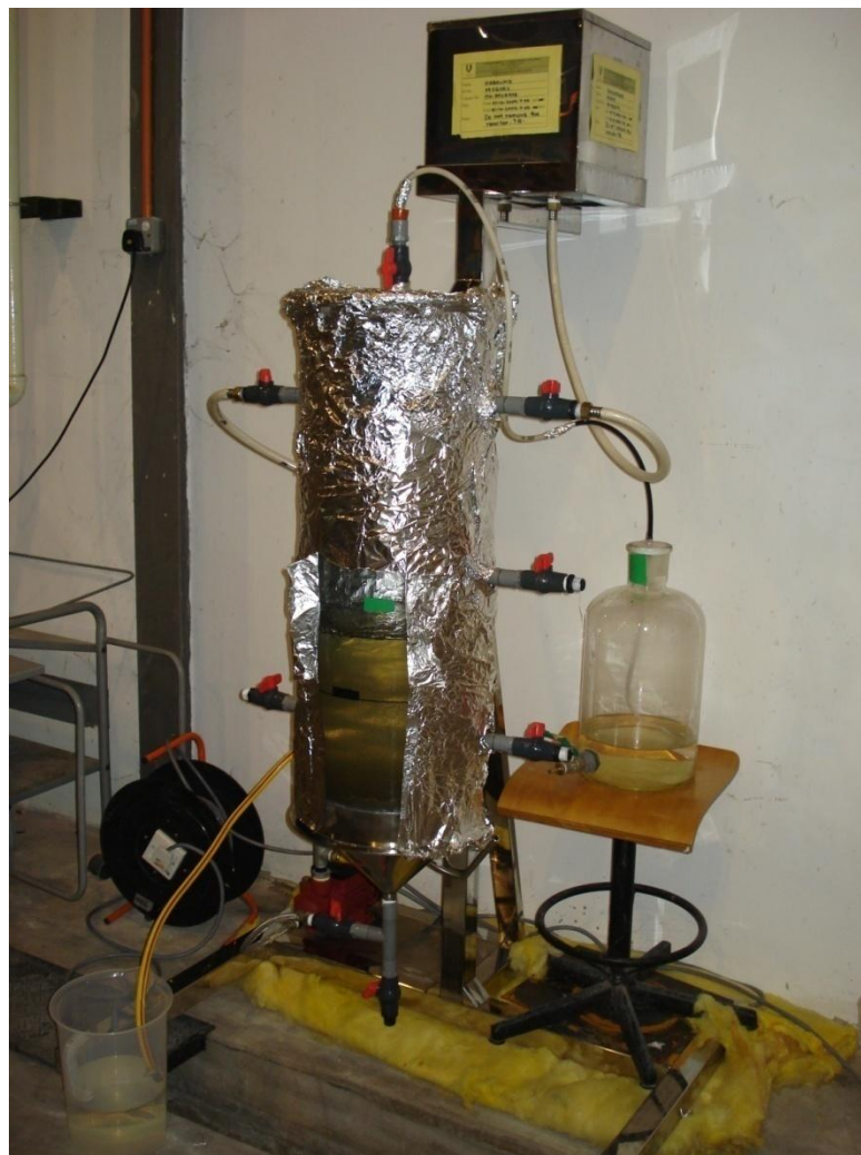
Figure 3.16: Feeder, Feeder Tank, Anaerobic Reactor of Membrane of Membrane Anaerobic System, 20 liter Displacement Bottle, and Effluent Collector.
