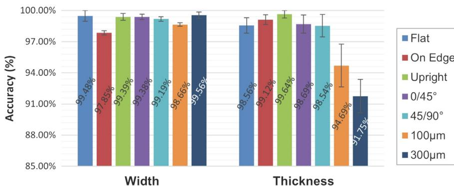
**Fig. 6.** Comparison among the average dimensional (width and thickness) accuracy of dog-bone test specimens manufactured in different print orientation, raster direction, and layer thickness.
