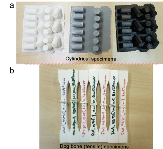
Fig. 2. (a) 3D-printed cylindrical specimens with different build orientations; (b) 3D-printed dog-bone tensile test specimens at various process parameters.
