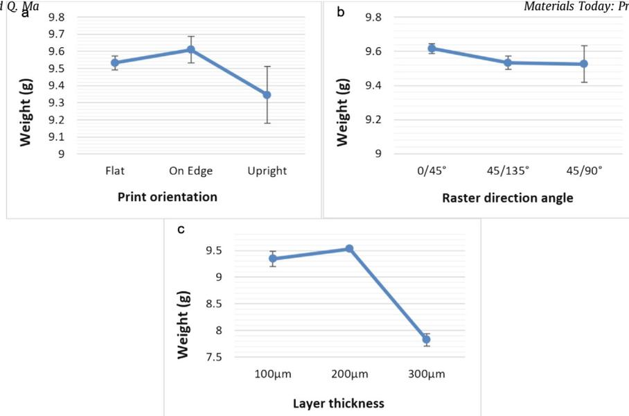
Fig. 7. Comparison among the average weight of dog-bone test specimens manufactured in different (a) print orientation; (b) raster direction angle, and (c) layer thickness.
