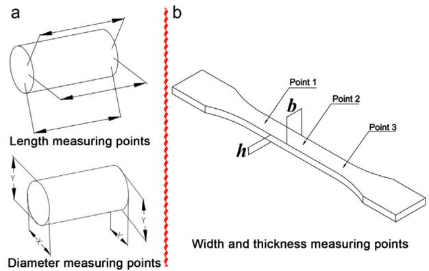
Fig. 3. (a) measurement positions for the length and diameter of cylindrical test samples; (b) measurement points for the width ( $b$ ) and thickness ( $h$ ) on the gauge section of the dog-bone tensile test specimen.
