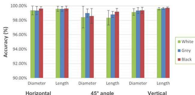
**Fig. 4.** Comparison among the average dimensional (diameter and length) accuracy of cylindrical test specimens manufactured in different print orientations and colors.
