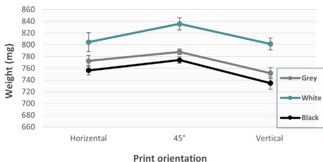
**Fig. 5.** Comparison among the average weight of cylindrical test specimens manufactured in different print orientations and colors.
