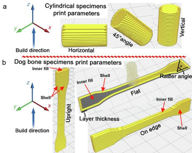
Fig. 1. (a) print orientations of cylindrical test specimens; (b) parameters used for printing dog-bone test specimens including print orientation, raster direction angle, and layer thickness.
