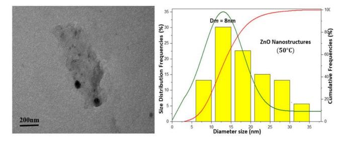
Figure 3: TEM image and size distribution chart of synthesised ZnO nanostructure synthesised at temperature 50°C.
