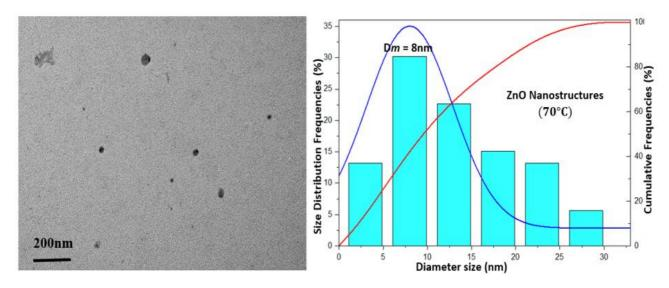
Figure 2: TEM image and size distribution chart of synthesised ZnO nanostructure synthesised at temperature 70°C.
