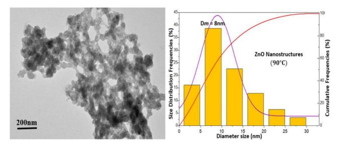
Figure 1: TEM image and size distribution chart of synthesised ZnO nanostructure synthesised at temperature 90°C.
