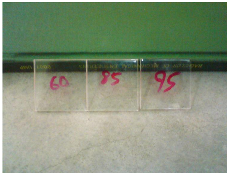
Figure 3.8: Samples of Acrylic with Different Power Levels
