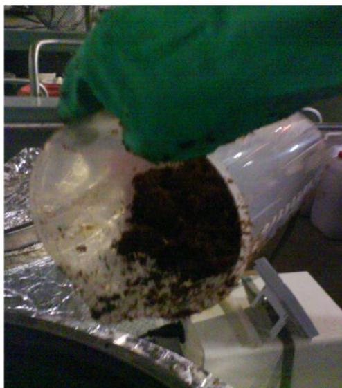
**Figure 3.7:** Pretreated sawdust (NaOH pretreatment) being introduced into membrane reactor.
