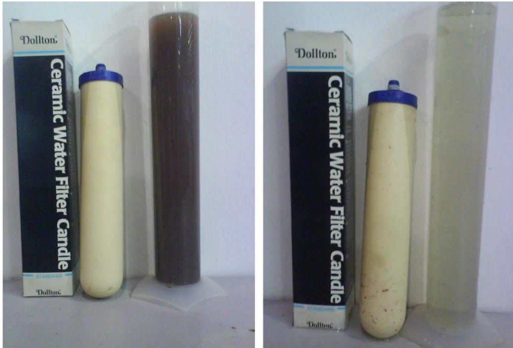
**Figure 3.11:** Membrane appearance and sample (a) before and (b) after filtration process.
