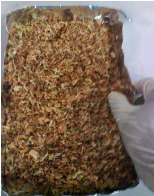
**Figure 3.2:** Sawdust taken from sawmill factory.
