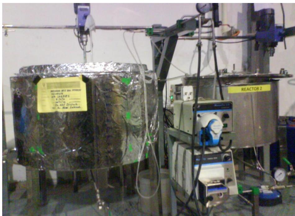
**Figure 3.9:** Membrane reactor system.
