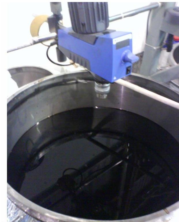
**Figure 3.5:** Sodium hydroxide (NaOH) pretreatment in membrane reactor.
