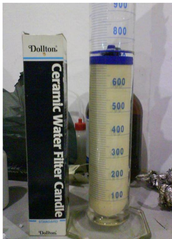
**Figure 3.13:** Chemical cleaning using 0.05M NaOH
