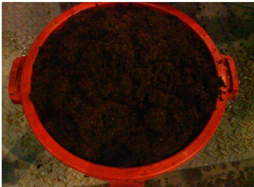
**Figure 3.6:** Sawdust (solid residue) after pretreatment process.
