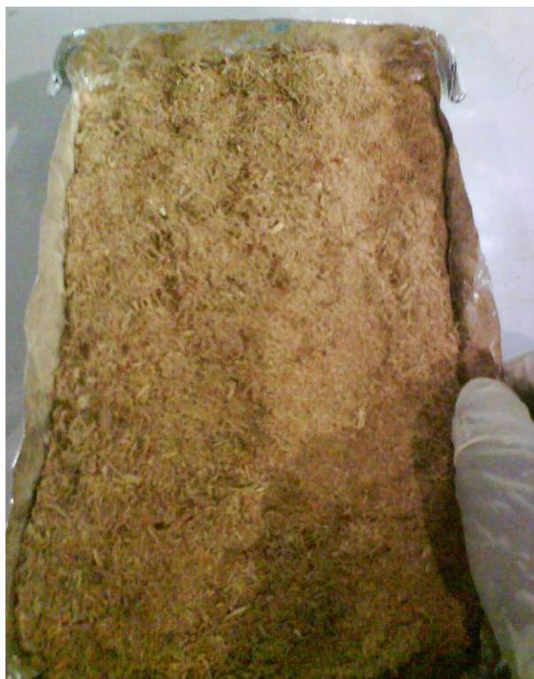
**Figure 3.4:** Sawdust after drying.
