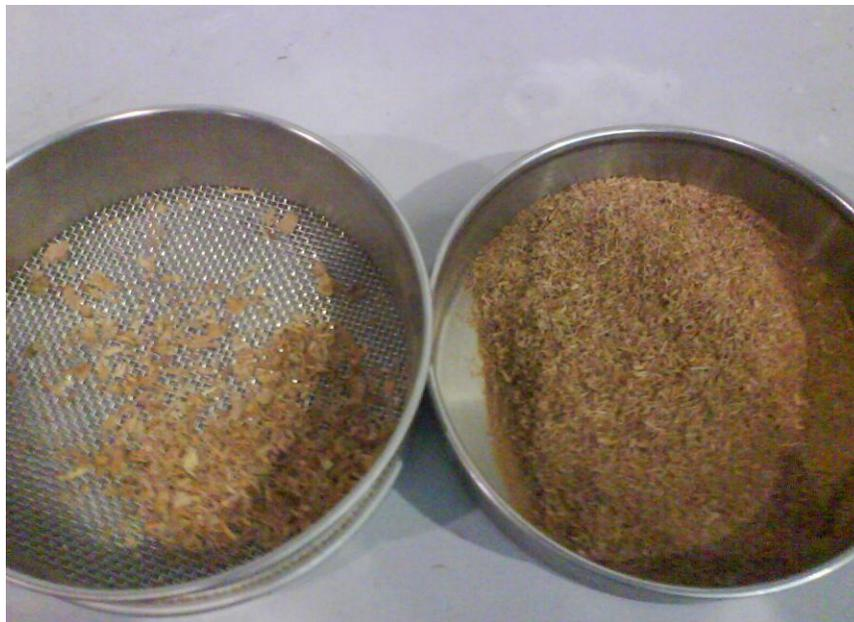
**Figure 3.3:** Sawdust after grinder and sieved.
