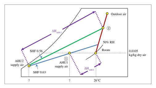
Figure 4. Determination of supply air temperature using psychrometric chart
