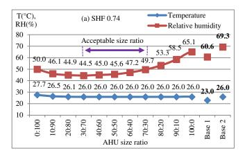
Figure 3. AHU acceptable size ratio
