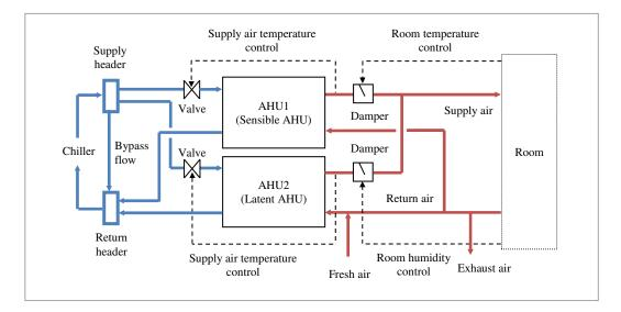
Figure 1. Schematic diagram of the proposed system
