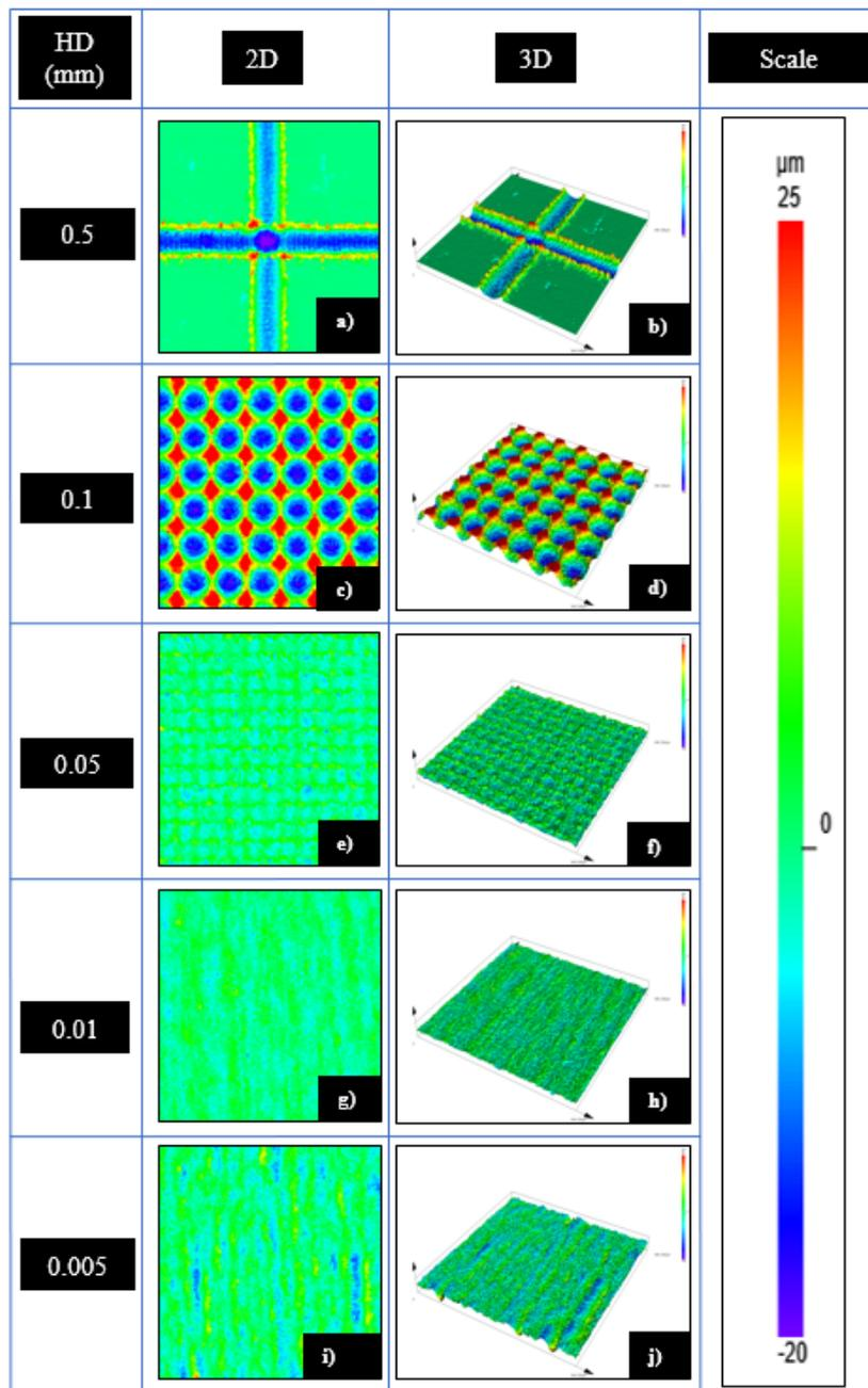
Figure 3. 2D overview of sample height image from laser scanning on each LSM sample with different hatching distance from 0.5 to 0.005 mm.
