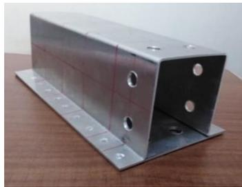
**Figure 1.** Top-hat crash box structure with spot-weld joint
