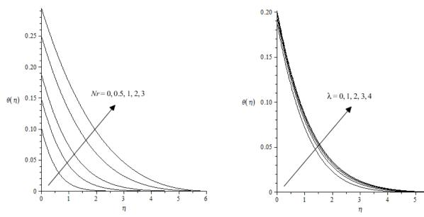
**Fig. 4.** Variation of temperature  $\theta(\eta)$  versus Nr
