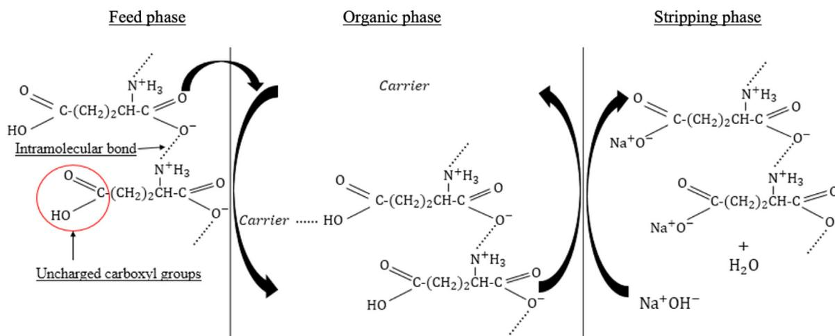
Fig. 5. Enrichment principle of GAs with carrier.
