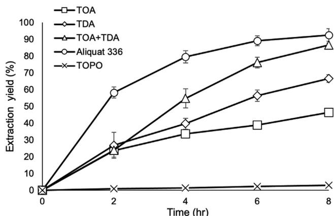
Fig. 6. Extraction yield of GA over time from aqueous solution by using 0.5 M of different carriers.
