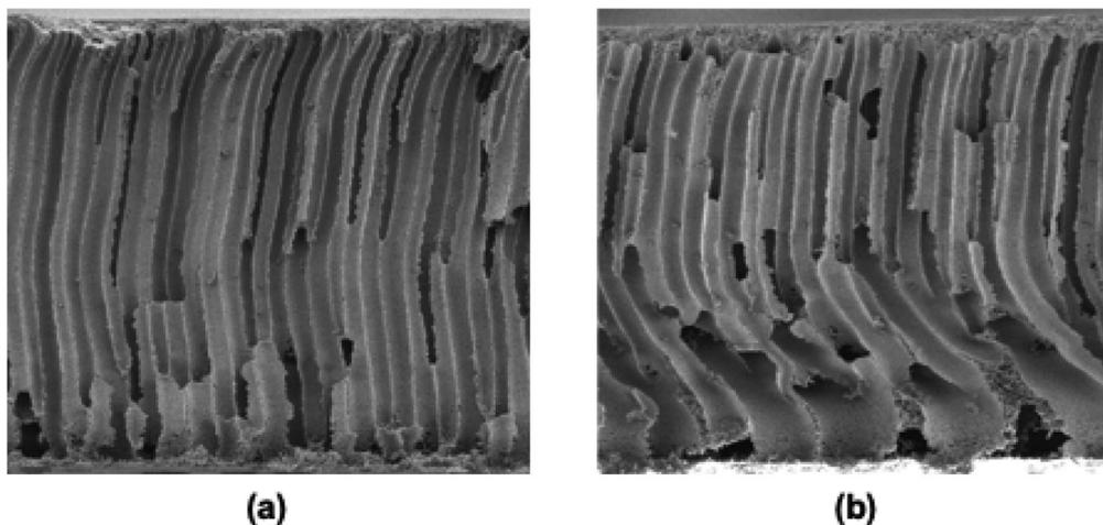
Fig. 1. Cross section of (a) pristine PES and (b) hybrid PES-graphene membrane.
