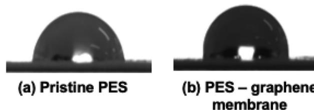
Fig. 2. Contact angle of the (a) pristine PES and (b) hybrid PES-graphene membrane.
