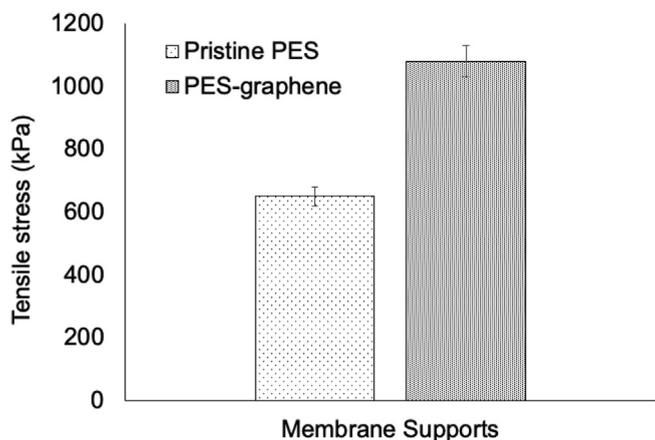
Fig. 3. Average stress to break value of pristine PES and PES-graphene membrane.
