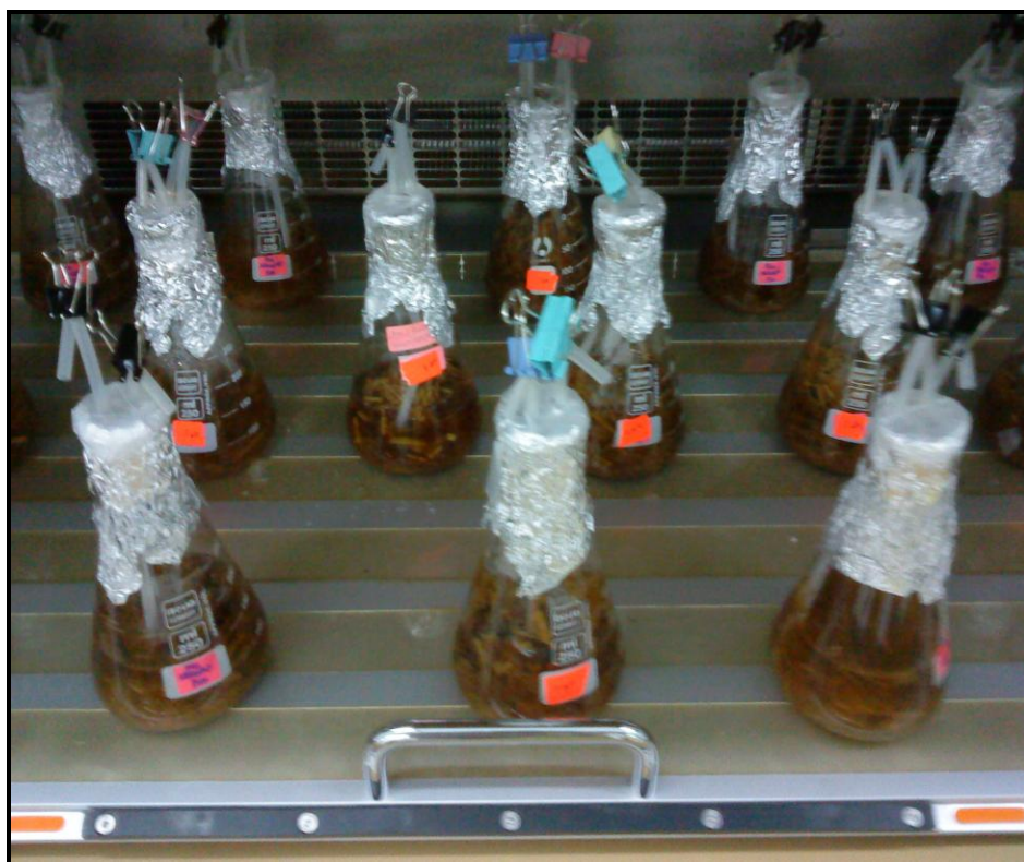
Figure 3.10: The shake flask incubated at 30°C and 150 rpm
