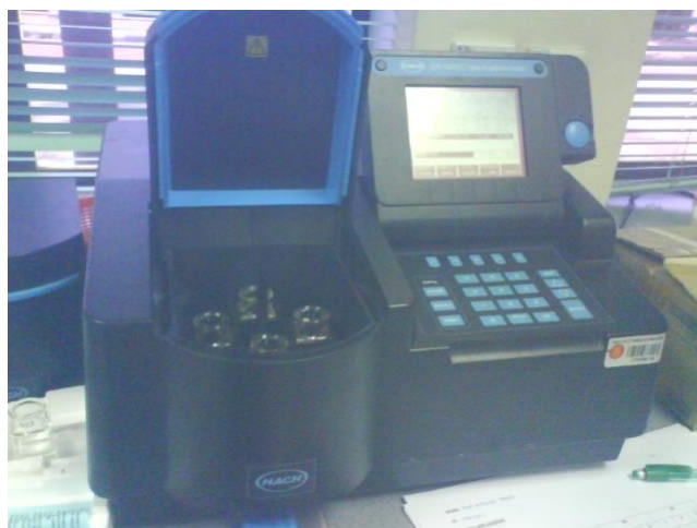
Figure A.2: HACH Spectrophotometer model DR/4000
