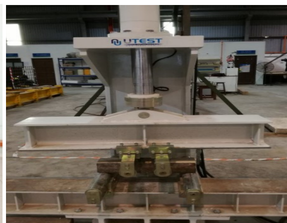
Figure 3. Automatic Flexural Test Machine
