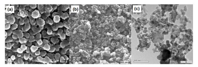
**Figure 3.** Various structures of surfactant-assisted photocatalysts: (a) raspberry-like; (b) rod-like; and (c) quasi-spherical. Adapted with permission from [65,67,68]. Copyright Elsevier and ESG.
