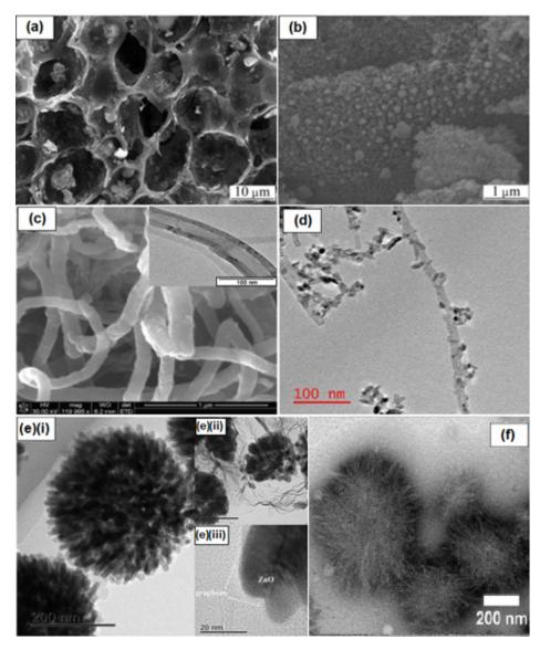
**Figure 5.** HRSEM images of (a) AC and (b) AC-supported Zr, (c) SEM image of functionalized CNT (inset: TEM), TEM images of (d) CNT/TiO<sub>2</sub> nanohybrids, (e) (i) ZnO nanospheres and (e) (ii) ZnO-graphene nanocomposites, (e) (iii) HRTEM of ZnO-graphene nanocomposites, and (f) TEM images of CQD/Fe<sub>3</sub>O<sub>4</sub>@mTiO<sub>2</sub>. Adapted with permission from [75,80–82]. Copyright Elsevier and ACS Publications.
