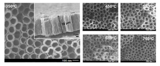
**Figure 2.** SEM images of reduced r-TiO<sub>2</sub> nanotube arrays prepared in annealing temperatures from 350 °C to 750 °C. Adapted with permission from [22]. Copyright Elsevier.
