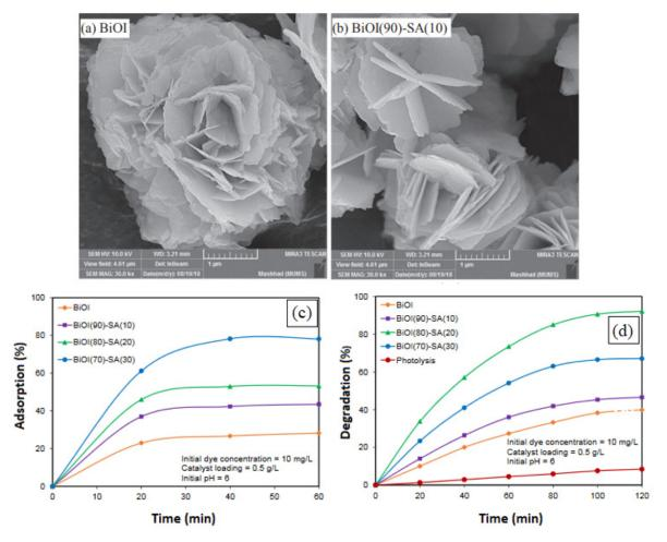
**Figure 6.** FESEM images of nanostructure flower-like photocatalysts: (a) BiOI; (b) silica aerogel/BiOI and effect of BiOI loading on Methylene Blue removal by BiOI and silica aerogel/BiOI photocatalysts: (c) adsorption; (d) degradation. Adapted with permission from [152]. Copyright Elsevier.
