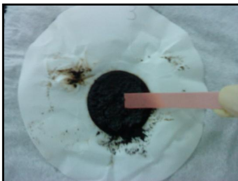
Step 5: Check pH then dry in oven
