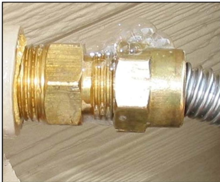
Figure 3.3: Gas leak test by using soap bubbles.
