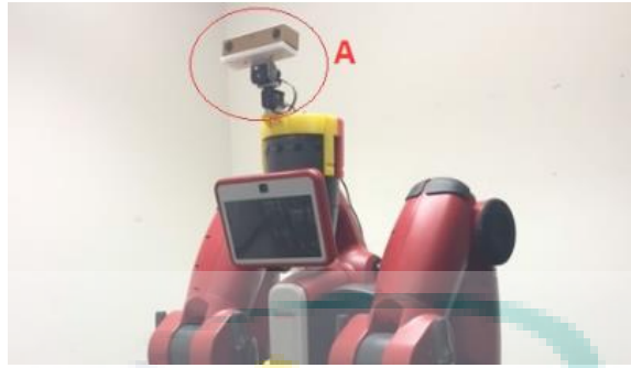
Figure 2.2 Bumblebee camera (Stereo head A) on 2 DOF robot Source: A. Cangelosi et al. (2016).
