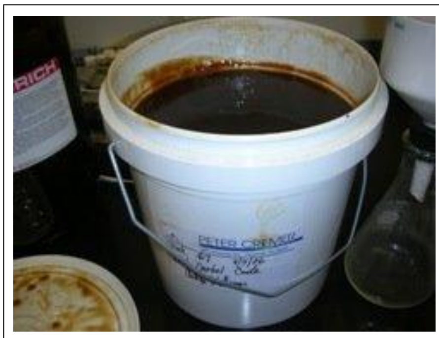
Figure 1.1 : Glycerol waste from biodiesel production process
