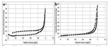
Figure 3  $N_2$  adsorption-desorption isotherm of (a) calcined commercial CaO and (b) calcined nano CaO
