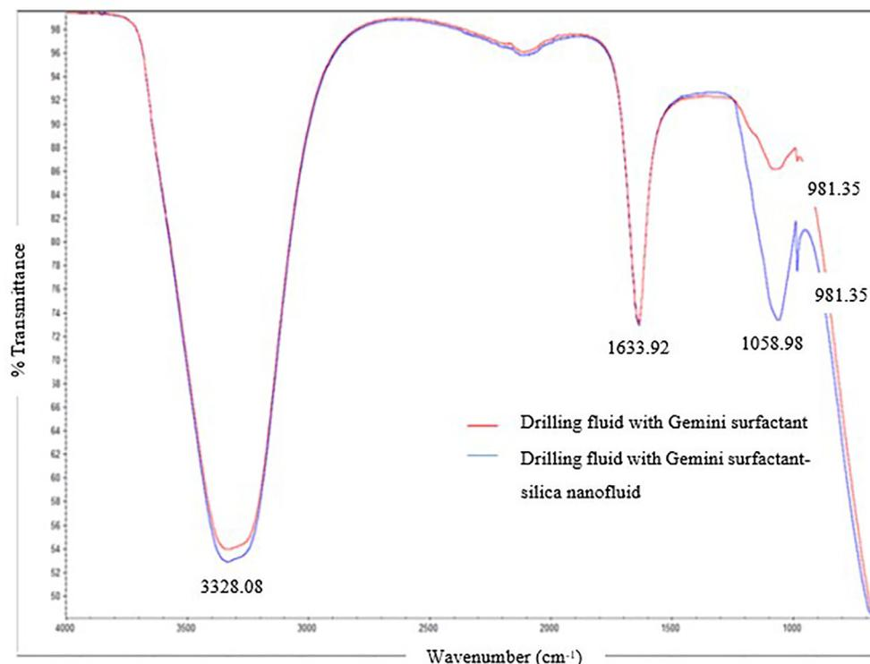
Fig. 1. FTIR spectra of the drilling fluid with and without silica nanofluid.
