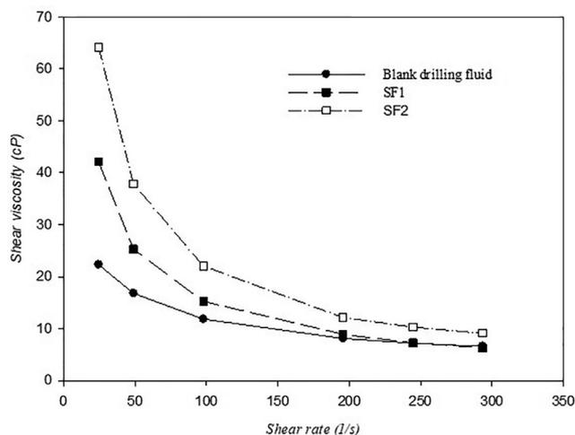
Fig. 2. Viscosity of the drilling fluid containing different surfactants.
