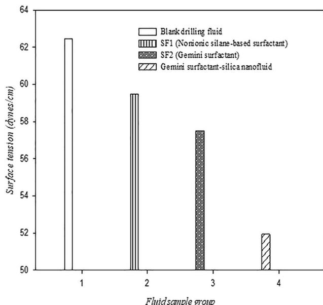
**Fig. 4.** Surface tension of drilling fluid containing different surfactants and with silica nanofluid.
