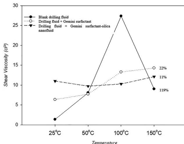
Fig. 3. Change in drilling fluid viscosity with increasing temperature.
