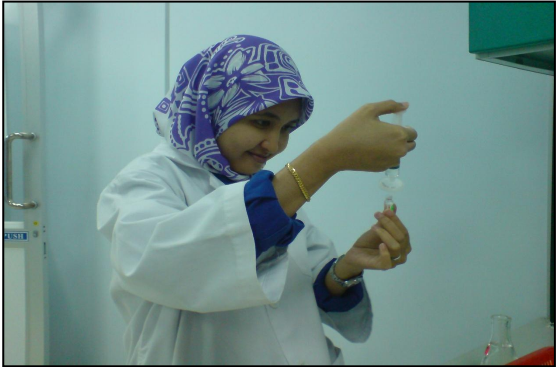
Figure 3.17 Filtration of Glucose Before Being Analyzed
