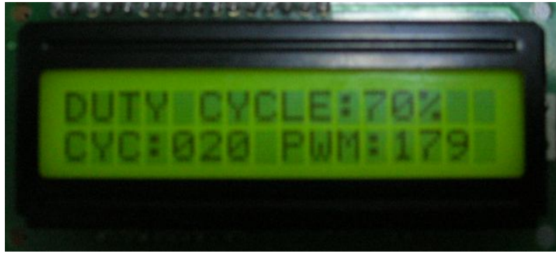
Figure 4.13: The information of duty cycle on the LCD
