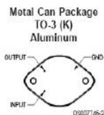
Bottom View Order Number LM7805CK, LM7812CK or LM7815CK See NS Package Number KC02A
