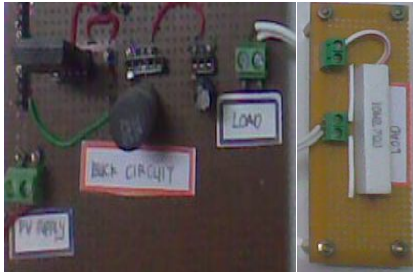
Figure 4.10: The complete buck converter circuit
