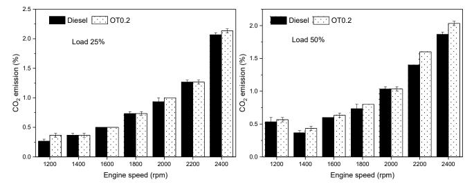
Figure 9. CO<sub>2</sub> emission at various engine speeds.
