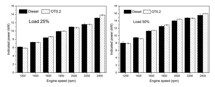
Figure 5. Indicated power at various engine speeds.
