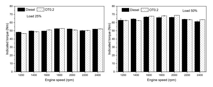
Figure 6. Indicated torque at various engine speeds.
