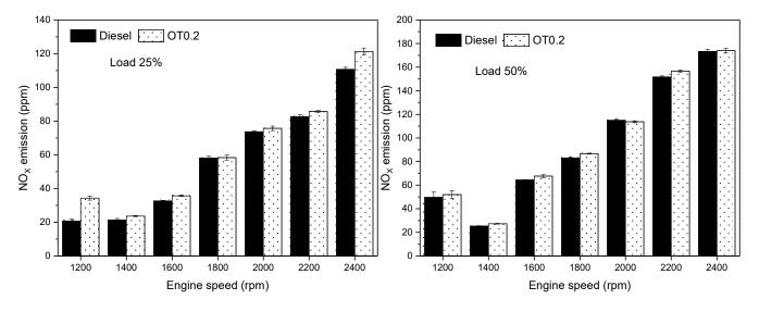
**Figure 10.**  $NO_X$  emission at various engine speeds.
