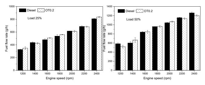
Figure 7. Fuel flow rate at various engine speeds.
