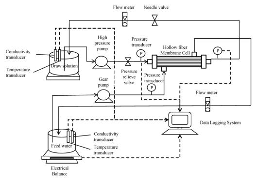
Figure 3. Schematic diagram of bench-scale PRO system [27].
