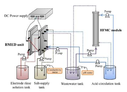
**Figure 7.** Schematic experimental setup of bipolar membrane electrodialysis and hollow fiber membrane contactor for ammonia capture from wastewater [39].
