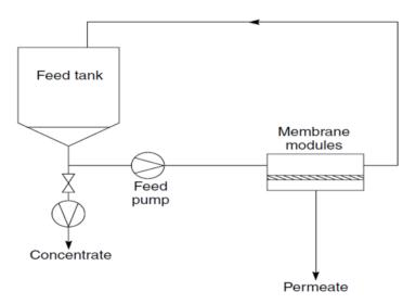
Figure 1. Schematic flow of a batch ultrafiltration process.
