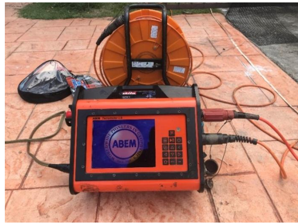
Figure 4. ABEM Terrameter LS2 and 200m cable
