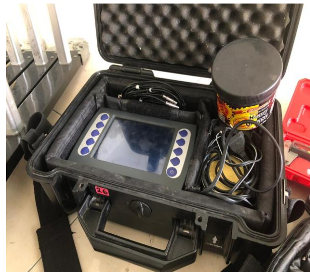
Figure 2. Ultrasonic Pulse Velocity Equipment
