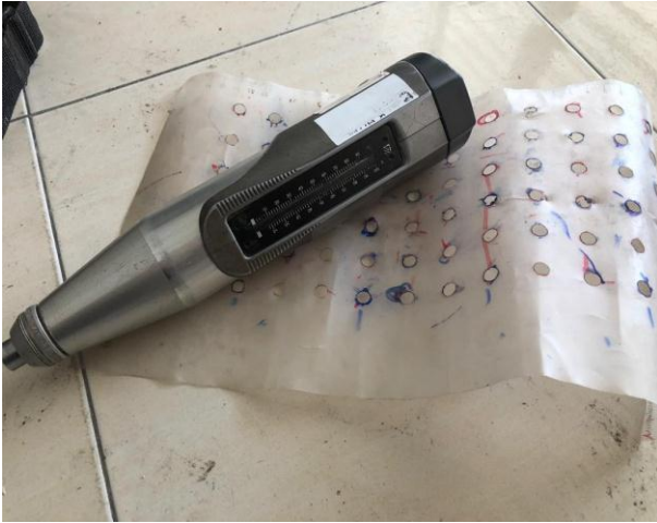
Figure 3. Rebound Hammer Equipment
