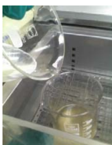
Figure 3.14: Methanol was added into heated jatropha oil process
