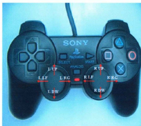
Figure 3.8: Joystick direction output
