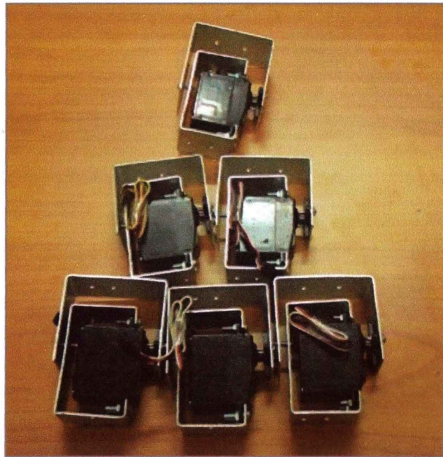
Figure 3.14: Connect the Connector Bracket with Servo Bracket
