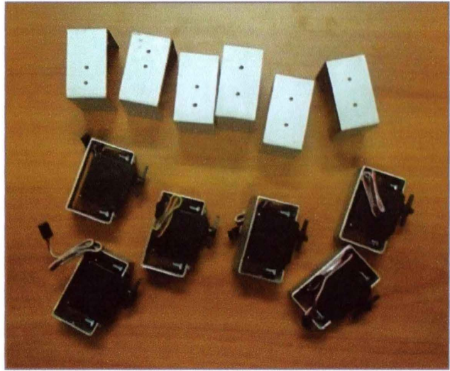
Figure 3.13: Mounting Servo Motor at the Servo Bracket
