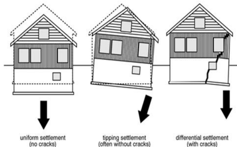
Figure 1.1 Settlement pattern of buildings on soft clay
