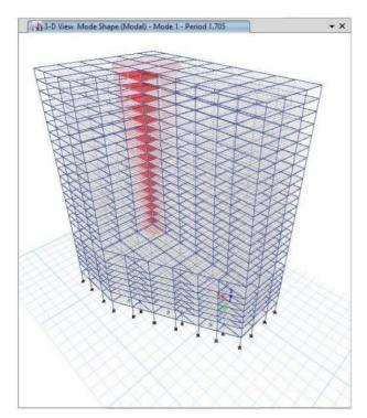
Figure 3. Mode shape 1 (building with shear wall)
