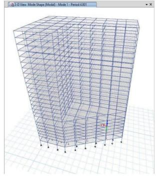
Figure 4. Mode shape 2 (building with no shear wall)
