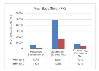
Figure 5. Maximum base shear in X direction
