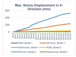
Figure 12. Maximum storey displacement in X direction
