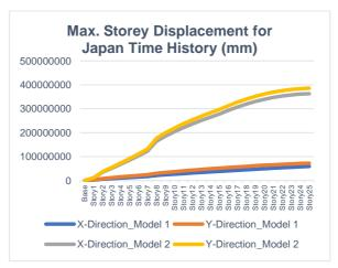
Figure 14. Maximum storey displacement for Japan time history
